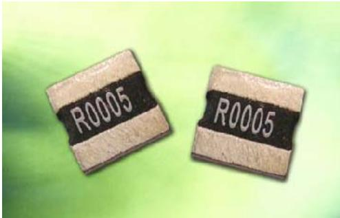
The CSS / CSSH Series is available in chip sizes 1206 - 0.5 watt, 2010 - 1 watt, 2512 - 2 watt and 3 watt, 2725 - 4 watt, and 2728 - 3 watt and 4 watt. TCR's range from 15 ppm to 50 ppm and tolerances down to 0.5% are available as standard product. This series is available in 7" reels with embossed tape and quantities of 1000 or 2000 pieces depending on size. Pricing varies with size, tolerance, and resistance value and ranges. Contact NAC for volume pricing.
