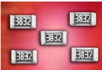
The RNCP Series resistors were developed with a high tolerance for harsh environments, including shock, vibration and temperature extremes with the goal of enhancing their performance and lifespan. The thin film technology provides high power handling, stability and low noise, giving them ideal characteristics for use in notebook computers, printers, scanners and test instruments.
