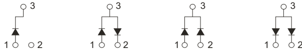
CDBT-40-HF Marking Code: 43 CDBT-40S-HF Marking Code: 44 CDBT-40C-HF Marking Code: 45 CDBT-40A-HF Marking Code: 46
