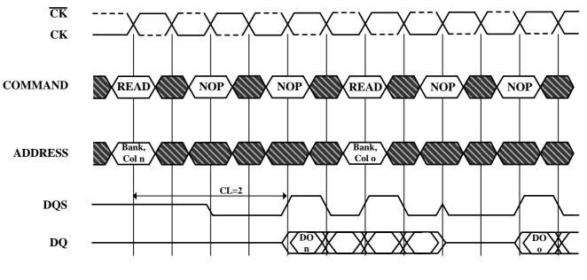
DO n (or o)=Data Out from column n (or column o) Burst Length=4 3 subsequent elements of Data Out appear in the programmed order following DO n (and following DO o)
