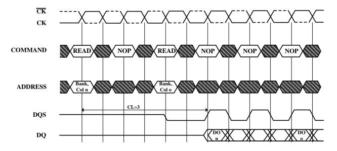
DO n (or o)=Data Out from column n (or column o) Burst Length=4 or 8 (if 4, the bursts are concatenated; if 8, the second burst interrupts the first) 3 subsequent elements of Data Out appear in the programmed order following DO n 3 (or 7) subsequent elements of Data Out appear in the programmed order following DO o Read commands shown must be to the same device
