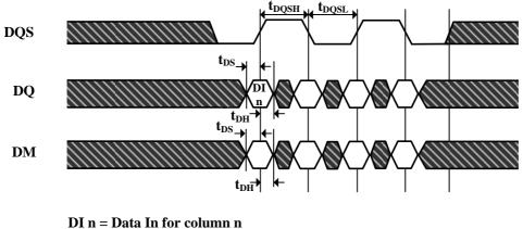
Burst Length = 4 in the case shown 3 subsequent elements of Data In are applied in the programmed order following DI n
