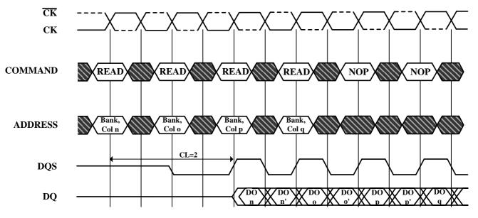
DO n, etc. =Data Out from column n, etc. n', etc. =the next Data Out following DO n, etc. according to the programmed burst order Burst Length=2,4 or 8 in cases shown. If burst of 4 or 8, the burst is interrupted Reads are to active rows in any banks
