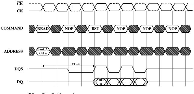
DO n = Data Out from column n Cases shown are bursts of 8 terminated after 4 data elements 3 subsequent elements of Data Out appear in the programmed order following DO n
