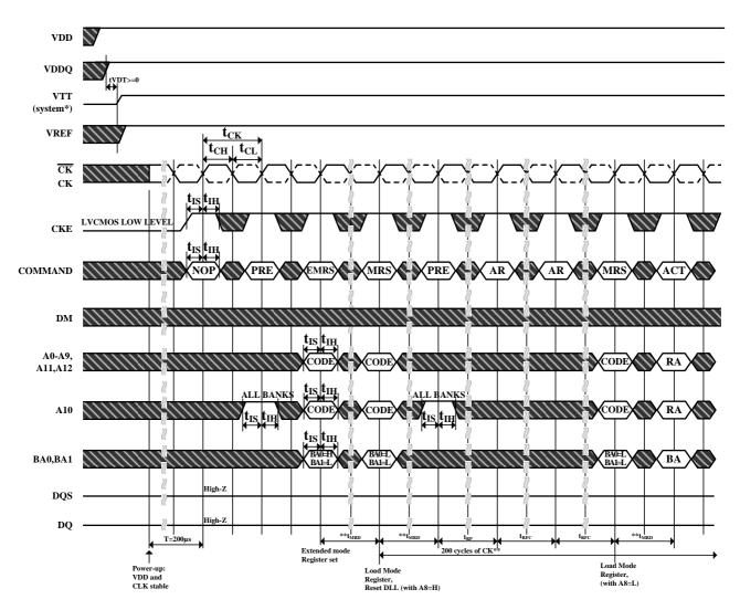
\*=VTT is not applied directly to the device, however tVTD must be greater than or equal to zero to avoid device latch-up. \*\* = tMRD is required before any command can be applied, and 200 cycles of CK are required before any executable command can be applied the two auto Refresh commands may be moved to follow the first MRS but precede the second PRECHARGE ALL command.
