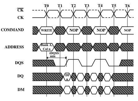
DI n = Data In for column n 3 subsequent elements of Data In are applied in the programmed order following DI n A non-interrupted burst of 4 is shown
