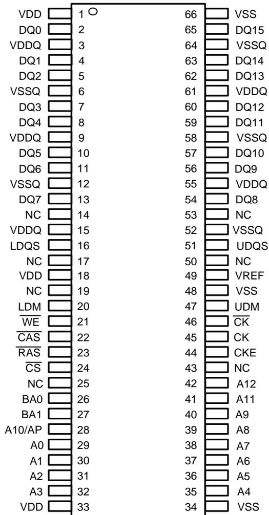
**Figure 1.1 Ball Assignment (Top View)**
