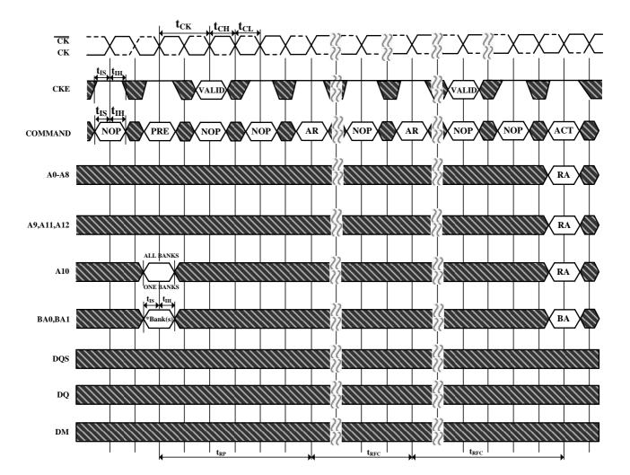
\* = "Don't Care", if A10 is HIGH at this point; A10 must be HIGH if more than one bank is active (i.e., must precharge all active banks) PRE = PRECHARGE, ACT = ACTIVE, RA = Row Address, BA = Bank Address, AR = AUTOREFRESH NOP commands are shown for ease of illustration; other valid commands may be possible after tRFC DM, DQ and DQS signals are all "Don't Care" /High-Z for operations shown
