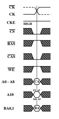
CA=Column Address BA=Bank Address EN AP=Enable Autoprecharge DIS AP=Disable Autoprecharge
