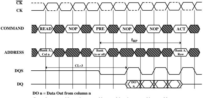
Cases shown are either uninterrupted bursts of 4, or interrupted bursts of 8 3 subsequent elements of Data Out appear in the programmed order following DO n
