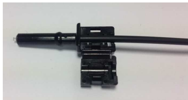
Figure 7. Cable and Connector Positioning
