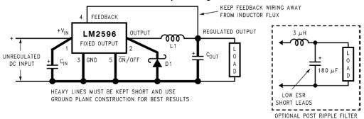
$C_{IN} = 470 \mu F$ , 50V,  $C_{OUT} = 220 \mu F$ , 25V (Aluminum Electrolytic Nichicon "PL Series"
