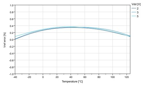
Figure 38-46. Internal 1.1V Reference vs. Temperature
