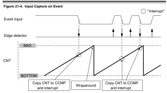
It is recommended to write '0' to the TCBn.CNT register when entering this mode from any other mode.
