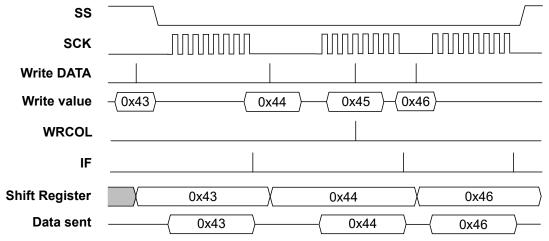
The figure above shows three transfers and one write to the DATA register while the SPI is busy with a transfer. This write will be ignored and the Write Collision Flag (WRCOL in SPIn.INTFLAGS) is set.
