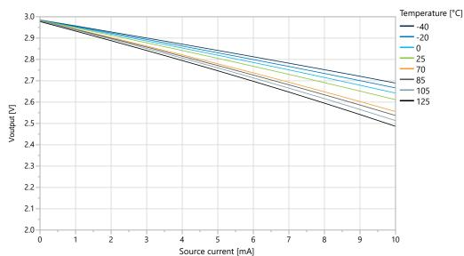
Figure 38-39. I/O Pin Output Voltage vs. Source Current (V<sub>DD</sub>=3.0V)
