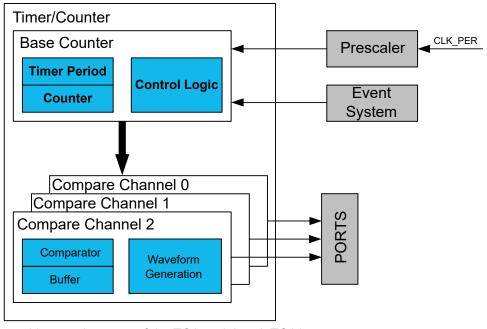
Figure 20-1. 16-bit Timer/Counter and Closely Related Peripherals
