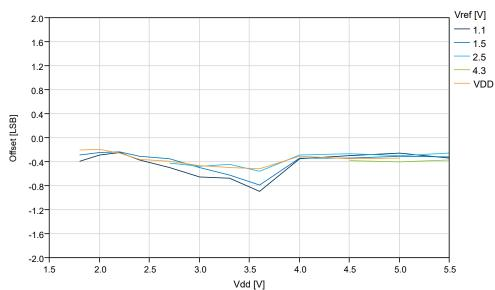
Figure 38-63. Offset Error vs. V<sub>DD</sub> (f<sub>ADC</sub>=115 ksps) at T=25°C, REFSEL = Internal Reference
