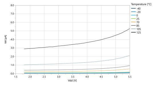
Figure 38-29. ATtiny3217 Power-Down Mode Supply Current vs. V<sub>DD</sub> (all functions disabled)
