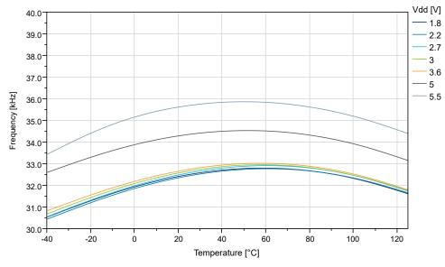
Figure 38-78. OSCULP32K Internal Oscillator Frequency vs. V<sub>DD</sub>
