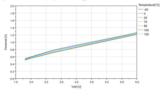
Figure 38-31. I/O Pin Input Threshold Voltage vs.  $V_{DD}$  (T=25°C)
