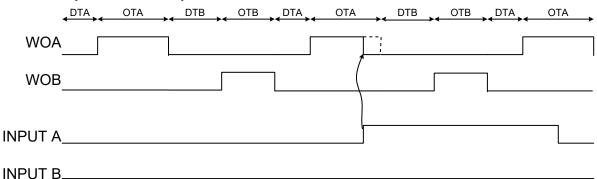
If Input mode 9 is used on input B and a positive input event occurs while in On-time B, the output will be OFF for the rest of the on-time.
