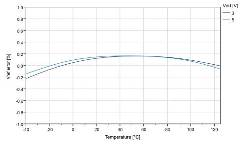
Figure 38-48. Internal 4.3V Reference vs. Temperature
