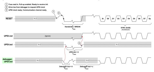
When the pull-up is detected, the debugger initiates the enable sequence by driving the line low for a duration of T<sub>Deb0</sub> to ensure that the line is released from the debugger before the UPDI enable sequence is done.
