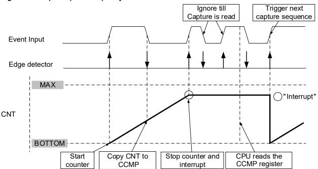
Figure 21-7. Input Capture Frequency and Pulse-Width Measurement
