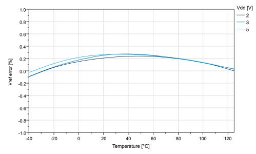
Figure 38-47. Internal 2.5V Reference vs. Temperature
