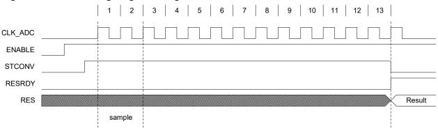
Both sampling time and sampling length can be adjusted using the Sample Delay bit field in Control D (ADC.CTRLD) and sampling the Sample Length bit field in the Sample Control register (ADC.SAMPCTRL). Both of these control the ADC sampling time in a number of CLK\_ADC cycles. This allows sampling high-impedance sources without relaxing conversion speed. See the register description for further information. Total sampling time is given by:
