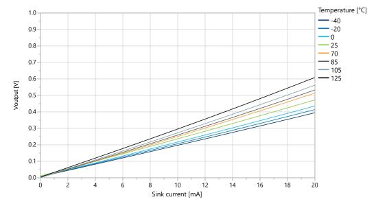
Figure 38-37. I/O Pin Output Voltage vs. Sink Current (T=25°C)
