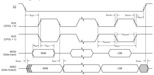
Figure 37-5. SPI - Timing Requirements in Slave Mode
