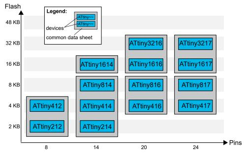
Devices with different Flash memory size typically also have different SRAM and EEPROM.
