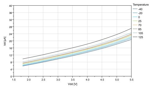
Figure 38-5. ATtiny1617 Active Supply Current vs. V<sub>DD</sub> (f=32 KHz OSCULP32K)
