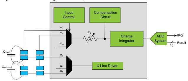
Figure 32-2. PTC Block Diagram Self Capacitance
