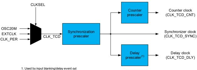
The TCD synchronizer clock is separate from the other module clocks enabling faster synchronization between the TCD domain and the I/O domain. The total prescaling for the counter is:
