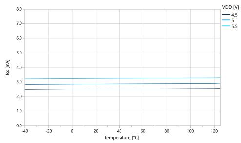
Figure 38-23. ATtiny3217 Idle Supply Current vs. Temperature (f=20 MHz OSC20M)
