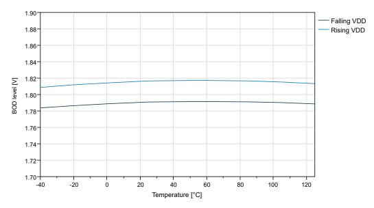
Figure 38-53. BOD Threshold vs. Temperature (Level 2.6V)
