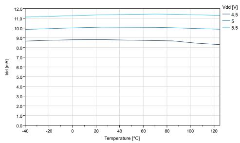
Figure 38-3. ATtiny1617 Active Supply Current vs. Temperature (f=20 MHz OSC20M)
