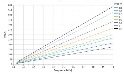
Figure 38-17. ATtiny3217 Active Supply Current vs. Frequency [0.1, 1.0] MHz at T=25°C
