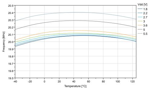
Figure 38-75. OSC20M Internal Oscillator: Frequency vs. Temperature
