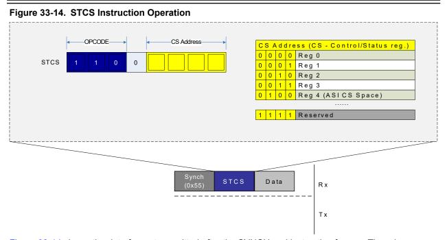
Figure 33-14 shows the data frame transmitted after the SYNCH and instruction frames. There is no response generated from the STCS instruction, as is the case for ST and STS.
