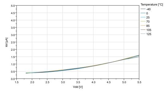
Figure 38-51. BOD Current vs.  $V_{DD}$  (Sampled BOD at 1 kHz)
