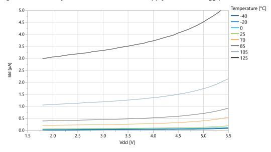
Figure 38-11. ATtiny1617 Power-Down Mode Supply Current vs. V<sub>DD</sub> (all functions disabled)
