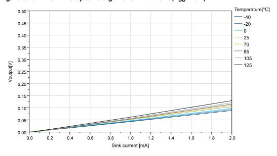
Figure 38-35. I/O Pin Output Voltage vs. Sink Current ( $V_{DD}$ =3.0V)
