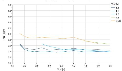
Figure 38-57. DNL Error vs.  $V_{DD}$  ( $f_{ADC}$ =115 ksps) at T=25°C, REFSEL = Internal Reference
