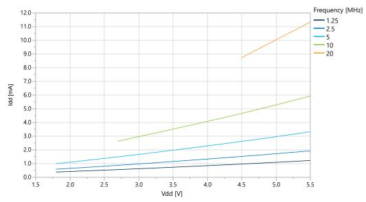
Figure 38-19. ATtiny3217 Active Supply Current vs. V<sub>DD</sub> (f=[1.25, 20] MHz OSC20M) at T=25°C
