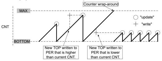
A counter wrap-around can occur in any mode of operation when up-counting without buffering. This is due to the fact that the TCAn.CNT and TCAn.PER registers are continuously compared: if a new TOP value is written to TCAn.PER that is lower than the current TCAn.CNT, the counter will wrap first, before a compare match happens.
