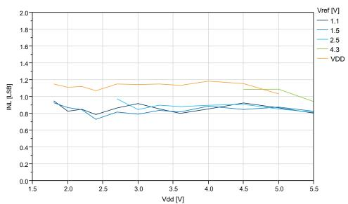
Figure 38-61. INL vs. V<sub>DD</sub> (f<sub>ADC</sub>=115 ksps) at T=25°C, REFSEL = Internal Reference
