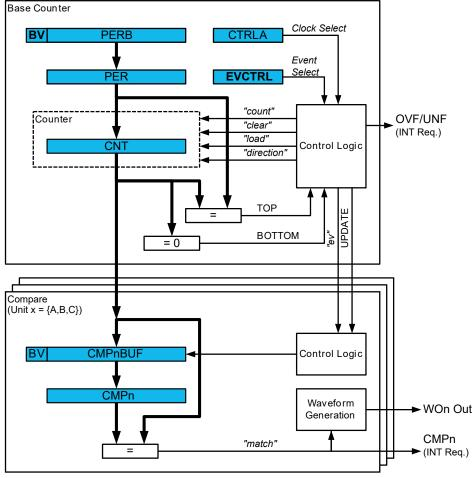
Figure 20-2. Timer/Counter Block Diagram
