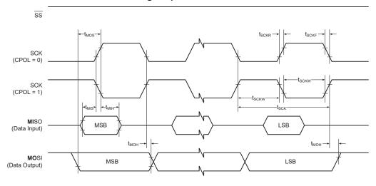
Table 37-19. USART in SPI Master Mode - Timing Characteristics
