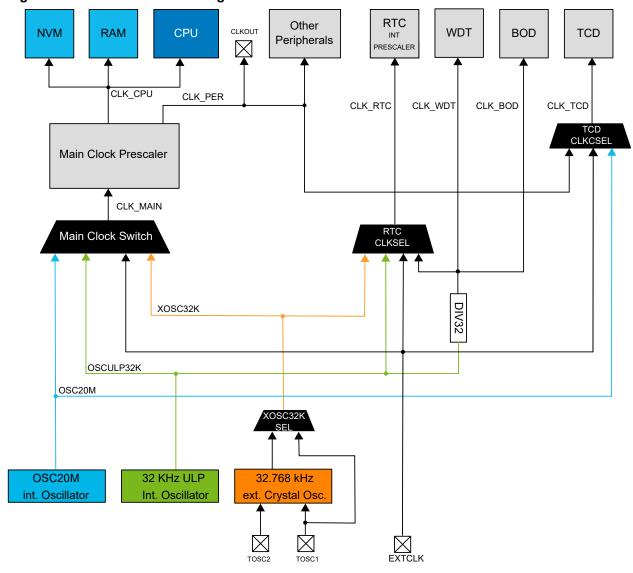
The clock system consists of the main clock and other asynchronous clocks:
