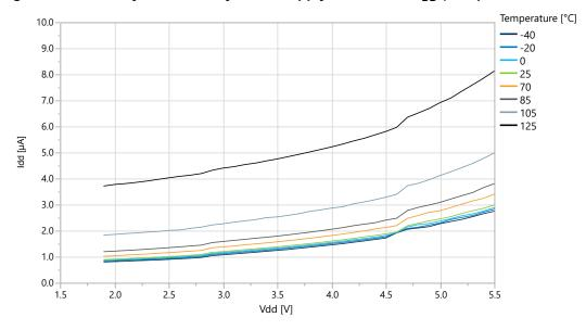
Figure 38-27. ATtiny3217 Standby Mode Supply Current vs. V<sub>DD</sub> (Sampled BOD Running at 1 kHz)
