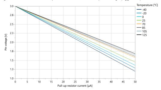
Figure 38-43. I/O Pin Pull-Up Resistor Current vs. Input Voltage (V<sub>DD</sub>=3.0V)
