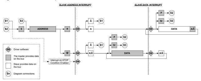
The number of interrupts generated is kept to a minimum by automatic handling of most conditions. Quick command can be enabled to auto-trigger operations and reduce software complexity.
