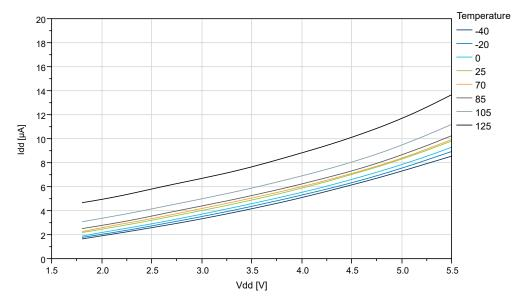
Figure 38-9. ATtiny1617 Idle Supply Current vs. V<sub>DD</sub> (f=32 KHz OSCULP32K)
