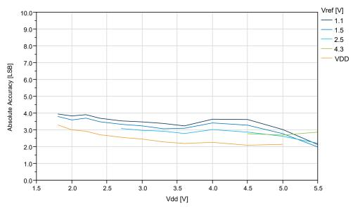
Figure 38-56. Absolute Accuracy vs.  $V_{ref}$  ( $V_{DD}$ =5.0V,  $f_{ADC}$ =115 ksps), REFSEL = Internal Reference
