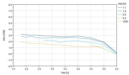
Figure 38-59. Gain Error vs.  $V_{DD}$  ( $f_{ADC}$ =115 ksps) at T=25°C, REFSEL = Internal Reference
