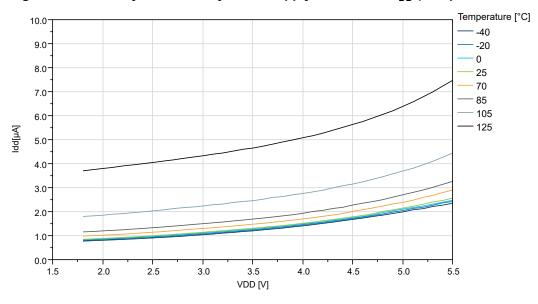
Figure 38-15. ATtiny1617 Standby Mode Supply Current vs. V<sub>DD</sub> (Sampled BOD Running at 1 kHz)
