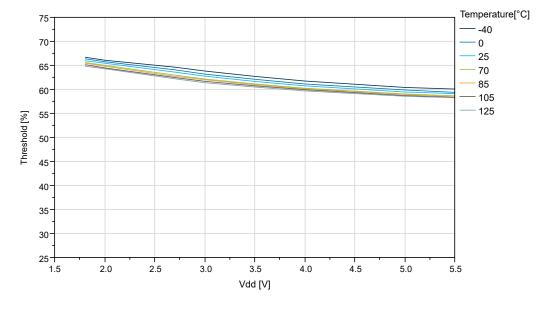
Figure 38-33. I/O Pin Input Threshold Voltage vs.  $V_{DD}$  ( $V_{IL}$ )
