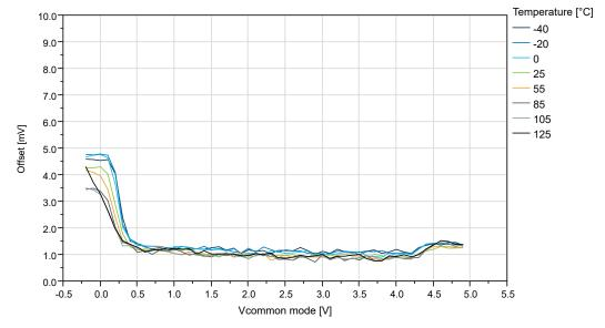
Figure 38-68. Offset vs.  $V_{CM}$  - 10 mV to 50 mV ( $V_{DD}$ =5V, T=25°C)
