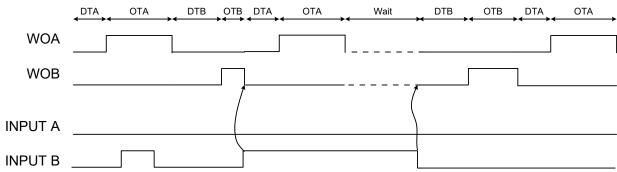
Input Mode 3: Stop Output, Execute Opposite Compare Cycle while Fault Active
