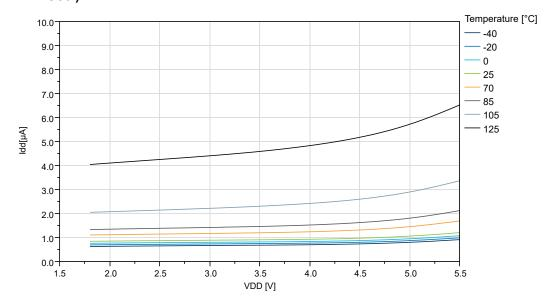
Figure 38-13. ATtiny1617 Standby Mode Supply Current vs.  $V_{DD}$  (RTC Running with Internal OSCULP32K)
