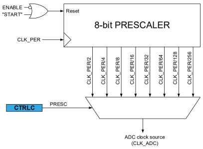
The ADC requires an input clock frequency between 50 kHz and 1.5 MHz for maximum resolution. If a lower resolution than 10 bits is selected, the input clock frequency to the ADC can be higher than 1.5 MHz to get a higher sample rate.
