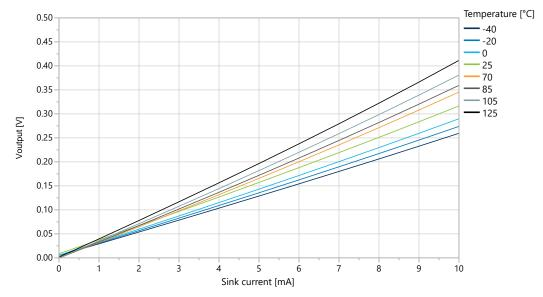
Figure 38-36. I/O Pin Output Voltage vs. Sink Current (V<sub>DD</sub>=5.0V)
