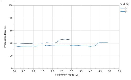
Figure 38-72. Propagation Delay vs.  $V_{CM}$  LPMODE Disabled, Rising Positive Input,  $V_{OD}$  = 30 mV (T=25°C)
