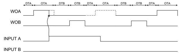
If Input mode 10 is used on input B and an input event occurs, the WOB will be OFF as long as the event lasts. If released during an on-time, it will be OFF for the rest of the on-time.
