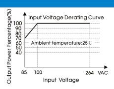
Note: ①Input voltage should be derated based on temperature derating when it is 85-264VAC/100-370VDC;
