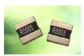
The CSS / CSSH Series is available in chip sizes 1206 - 0.5 watt, 2010 - 1 watt, 2512 - 2 watt and 3 watt, 2725 - 4 watt, and 2728 - 3 watt and 4 watt. TCR's range from 15 ppm to 50 ppm and tolerances down to 0.5% are available as standard product. This series is available in 7" reels with embossed tape and quantities of 1000 or 2000 pieces depending on size. Pricing varies with size, tolerance, and resistance value and ranges. Contact NAC for volume pricing.
