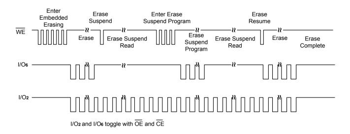
Note: Both I/Os and I/O2 toggle with OE or CE. See the text on I/Os and I/O2 in the section "Write Operation Statue" for more information.
