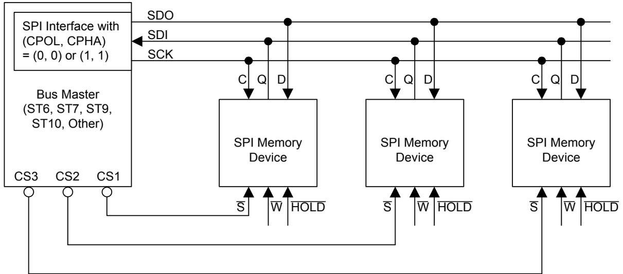
Note: The Write Protect ( $\overline{W}$ ) and Hold ( $\overline{HOLD}$ ) signals should be driven, High or Low as appropriate.
