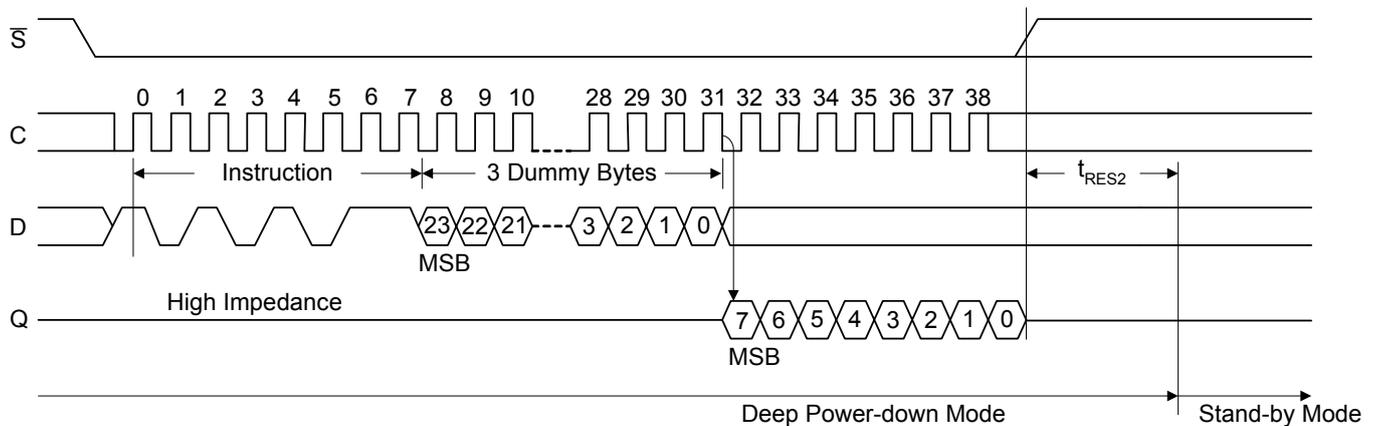
Note: The value of the 8-bit Electronic Signature, for the A25L80P, is 13h.
