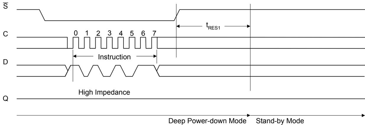
Driving Chip Select ( $\overline{S}$ ) High after the 8-bit instruction byte has been received by the device, but before the whole of the 8-bit Electronic Signature has been transmitted for the first time (as shown in Figure 16.), still insures that the device is put into Stand-by Power mode. If the device was not previously in the Deep Power-down mode, the transition to the Stand-by Power mode is immediate. If the device was
