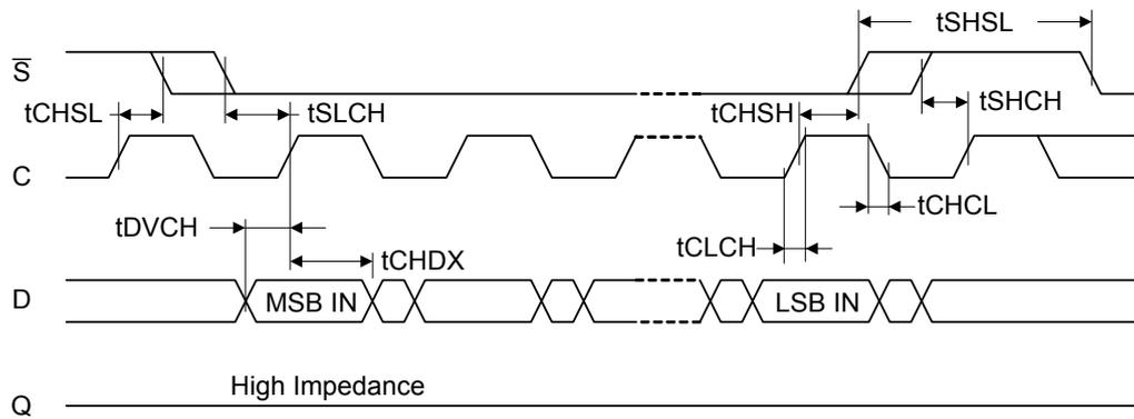
**Figure 20. Write Protect Setup and Hold Timing during WRSR when SRWD=1**
