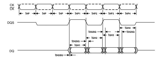
thP is the half cycle pulse width for each half cycle clock. thP is referenced to the clock duty cycle only and not to the data strobe (DQS) duty cycle.
