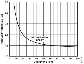
Figure 12. Propagation Delay vs. Input Overdrive
