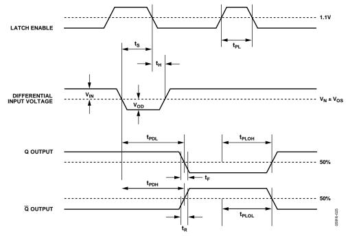
Figure 2. System Timing Diagram
