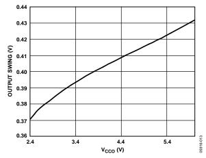
Figure 14. LVDS Output Swing vs. Vcco (V)
