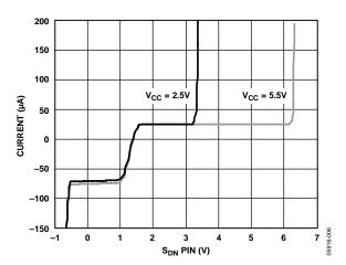
Figure 6. S<sub>DN</sub> Pin Current vs. Voltage
