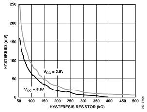
Figure 20. Hysteresis vs. R<sub>HYS</sub> Control Resistor
