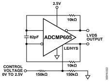
Figure 24. Voltage-Controlled Oscillator
