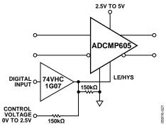
Figure 23. Hysteresis Adjustment with Latch
