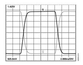
Figure 15. 50 MHz Output Voltage Waveform at  $V_{CCO} = 2.5 \text{ V}$
