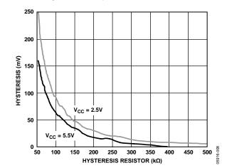
Figure 10. Hysteresis vs. Hysteresis Resistor
