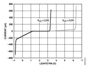
Figure 5. LE/HYS Pin Current vs. Voltage
