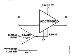
Figure 26. Hysteresis Adjustment with Latch
