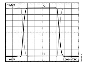
Figure 16. 50 MHz Output Voltage Waveform at  $V_{CCO} = 5 V$
