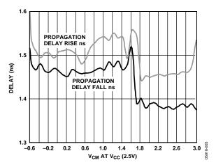
Figure 13. Propagation Delay vs. Input Common-Mode Voltage
