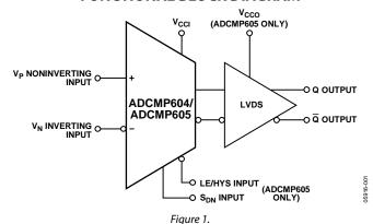
A flexible power supply scheme allows the devices to operate with a single 2.5 V positive supply and a -0.5 V to +2.7 V input signal range up to a 5.5 V positive supply with a -0.5 V to +5.7 V input signal range. Split input/output supplies, with no sequencing restrictions on the ADCMP605, support a wide input signal range with greatly reduced power consumption.
