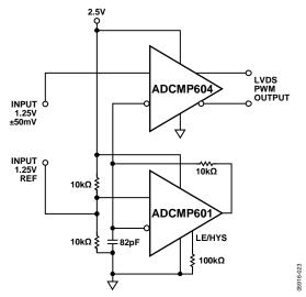
Figure 25. Oscillator and Pulse-Width Modulator
