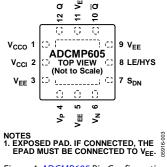
Figure 4. ADCMP605 Pin Configuration
