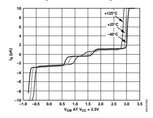
Figure 7. Input Bias Current vs. Input Common-Mode Voltage
