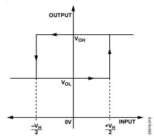
Figure 19. Comparator Hysteresis Transfer Function
