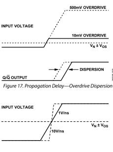
Figure 18. Propagation Delay—Slew Rate Dispersion
