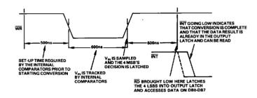
Figure 3. Operating Sequence (WR-RD Mode)
