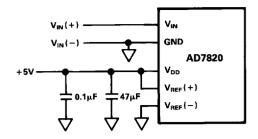
Figure 7a. Power Supply as Reference
