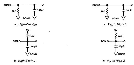
Figure 1. Load Circuits for Data Access Time Test
