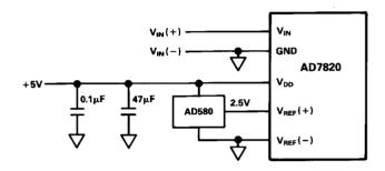
Figure 7b. External Reference 2.5V Full-Scale
