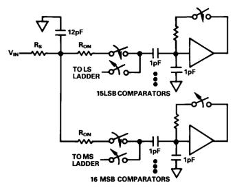
Figure 8a. AD7820 Equivalent Input Circuit
