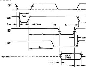
Figure 5a. WR-RD Mode (t<sub>RD</sub>>t<sub>INTL</sub>)
