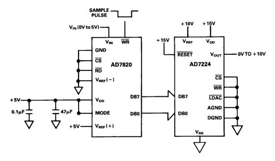
Figure 13. Fast Infinite Sample-and-Hold
