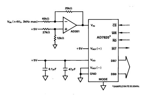
Figure 11. Telcom A/D Converter
