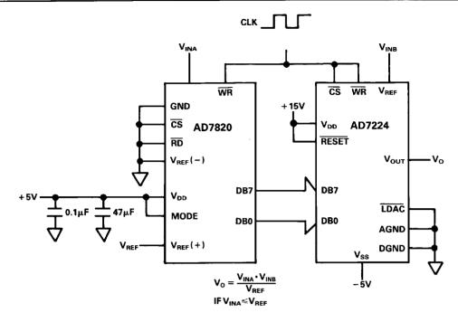
Figure 12. 8-Bit Analog Multiplier
