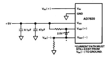
Figure 7c. Input Not Referenced to GND
