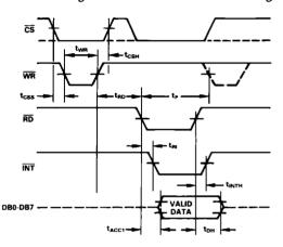
Figure 5b. WR-RD Mode (t<sub>RD</sub><t<sub>INTL</sub>)
