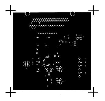
Figure 13. Printed Circuit Board Ground Layer
