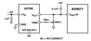
Figure 9. Using the AD780 Voltage Reference
