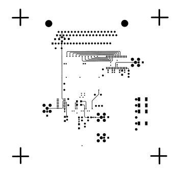
Figure 15. Printed Circuit Board Bottom Side Copper
