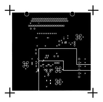
Figure 14. Printed Circuit Board "Split" Power Layer
