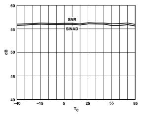
TPC 7. Differential SNR vs.  $T_C$ :  $f_{IN} = 10.3 \text{ MHz}$
