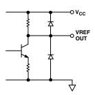
Figure 6. Equivalent Reference Output Circuit
