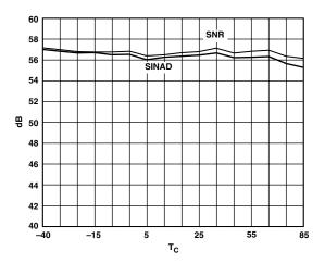
TPC 8. Single-Ended SNR vs.  $T_C$ :  $f_{IN} = 10.3 \text{ MHz}$
