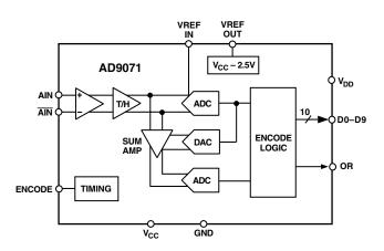
interfacing with 3.3 V or 5 V logic. An out-of-range output (OR) is available that indicates a conversion result is outside the operating range. The output data are held at saturation levels during an out-of-range condition.
