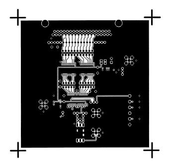
Figure 12. Printed Circuit Board Top Side Copper
