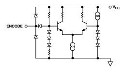
Figure 4. Equivalent Encode Input Circuit
