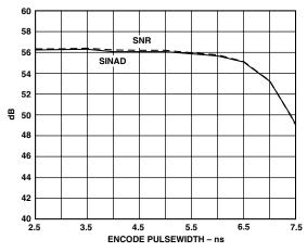
TPC 9. SNR vs. Clock Pulsewidth ( $t_{EH}$ ):  $f_{IN} = 10.3 \text{ MHz}$
