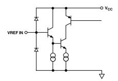
Figure 3. Equivalent Reference Input Circuit
