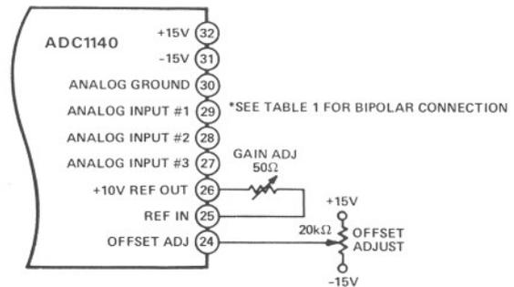
Figure 3. Offset and Gain Calibration
