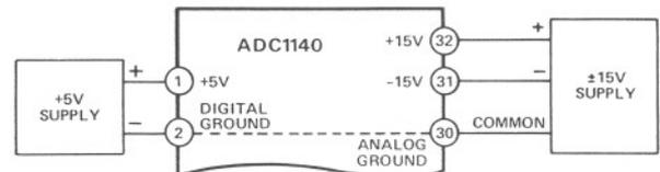
Figure 4. Power Supply and Grounding Techniques
