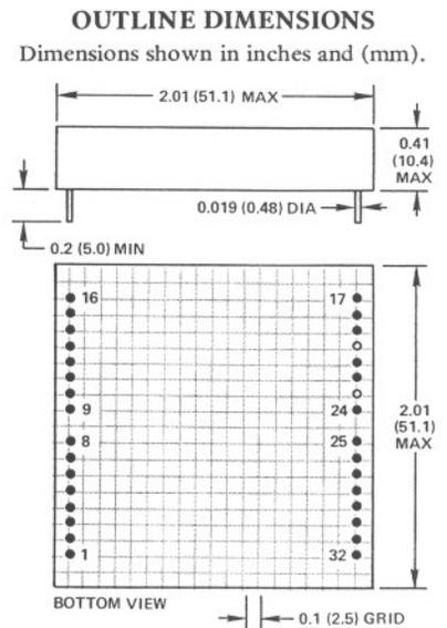
TERMINAL PINS INSTALLED ONLY IN SHADED HOLE LOCATIONS.
