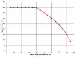
Ripple current versus actively cooled bus temperature for 10,000 hour life for continuous operation at 450V.
