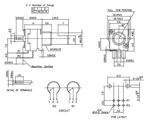
Model P09xP (Side Adjust, PCB pins, with Push-Lock, up to 2 gangs)
