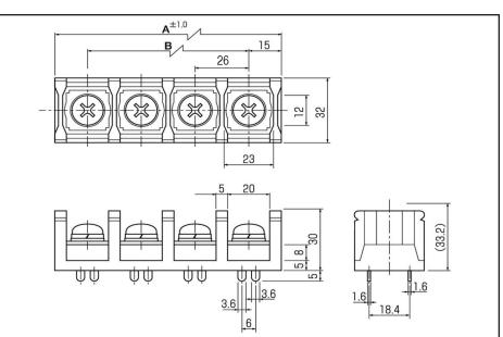
BlockMaster Electronics' new OTB-1500 series is a highpower PC board, barrier-style terminal block. This block allows you to terminate up to 100 AMPS per position. It has very heavy-duty PC terminals.
