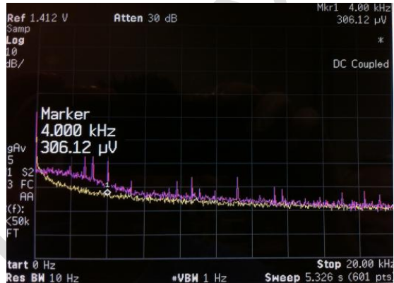
Voltage noise Density from 0.1Hz to 20 KHz (purple: with compensation; yellow: without compensation) (real value = measured value – 60dB)
