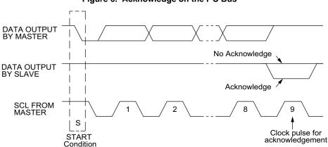
Figure 6. Acknowledge on the I<sup>2</sup>C Bus
