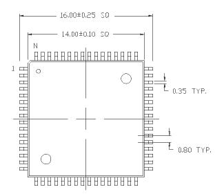
DIMENSIONS IN MILLIMETERS LEAD COPLANARITY 0.102 MAX.
