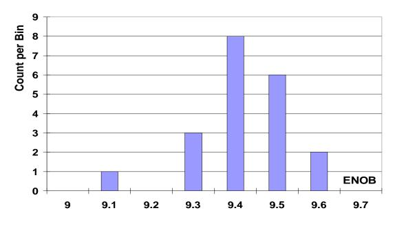
Figure 9: ENOB distribution measured at 25°C on 20 samples from 2 different wafer batches External CK=200kHz; 13.1kS/s
