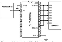
Figure 14. Left-justified 8-bit data bus.
