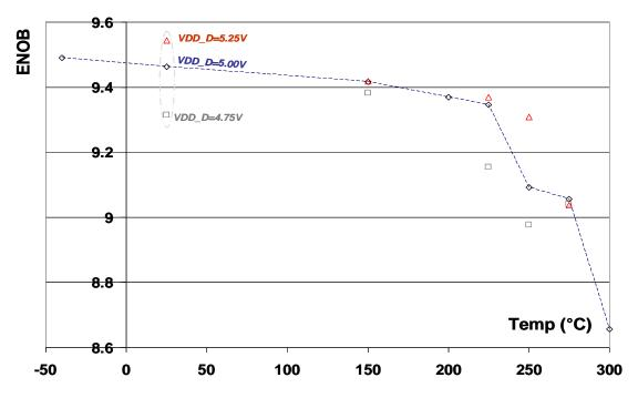
Figure 7: Typical ENOB over temperature; VDDD=4.75V; 5V; 5.25V
