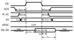
Figure 13. Read cycle timing.
