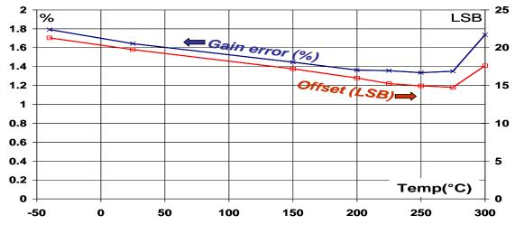
Figure 4: Typical Gain Error (%) and Offset (LSB) over temperature in [0...5]V range. External CK=200kHz
