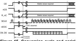
Figure 15. Conversion cycle and serial read protocol.
