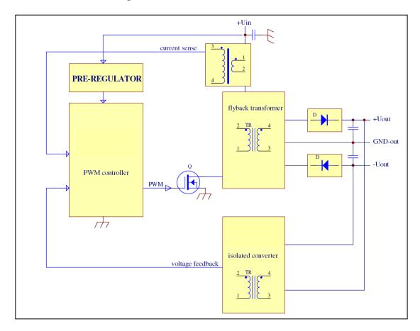
STROMBOLI® DC-DC Converter Technology is based on a flyback architecture which provides isolation capability, easy way to generate multiple outputs while keeping good regulation on all outputs. The same architecture is used to cover both input voltage ranges.
