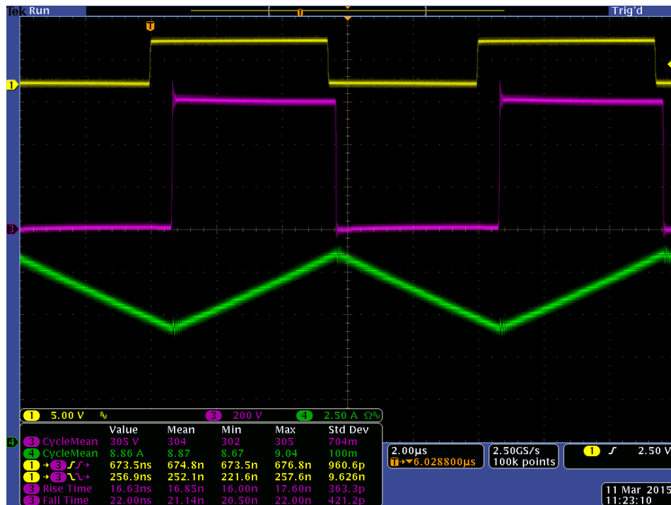
Figure 15: DC-DC operation at 100 kHz (CH1: PWM_L, CH3: half-bridge output voltage, CH4: Iload)
