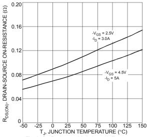
Fig. 6 On-Resistance Variation with Temperature
