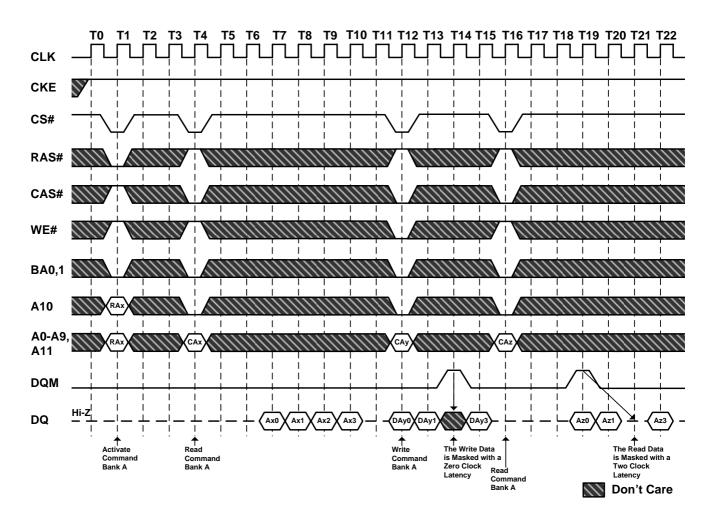
Figure 32.1. Interleaving Column Read Cycle (Burst Length=4, CAS# Latency=2)
