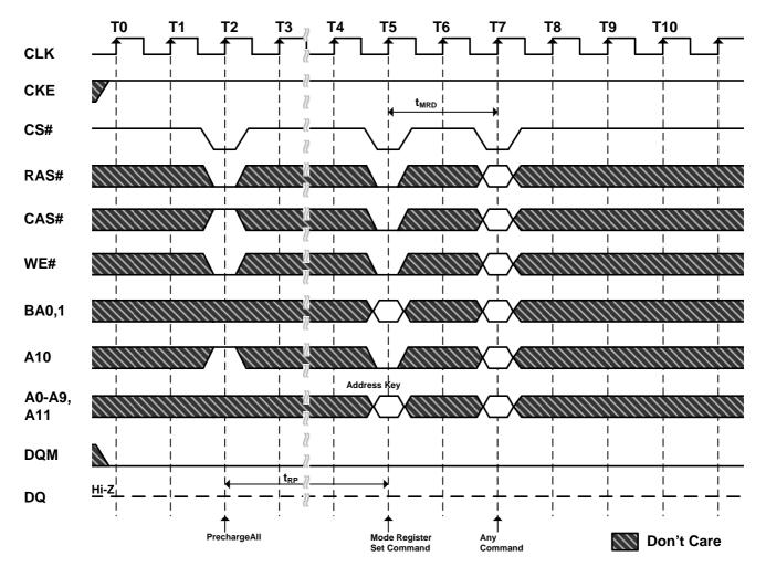
Figure 15. Mode Register Set Cycle
