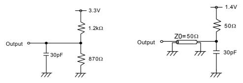
Figure 18.1 LVTTL D.C. Test Load (A)
