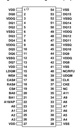
Figure 1.2 Ball Assignment (Top View)
