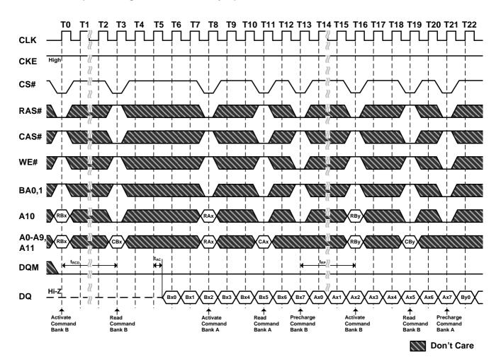
Figure 30. Random Row Write (Interleaving Banks)
