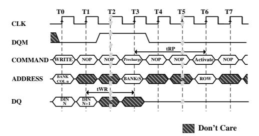
Note: The DQMs can remain low in this example if the length of the write burst is 1 or 2.
