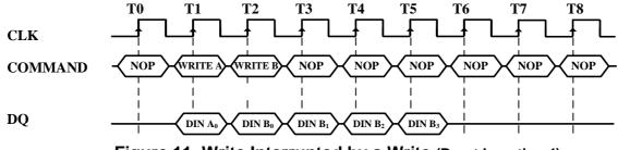
Figure 11. Write Interrupted by a Write (Burst Length = 4)
