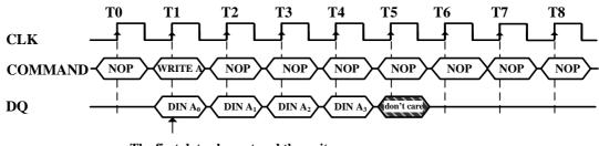
The first data element and the write are registered on the same clock edge
