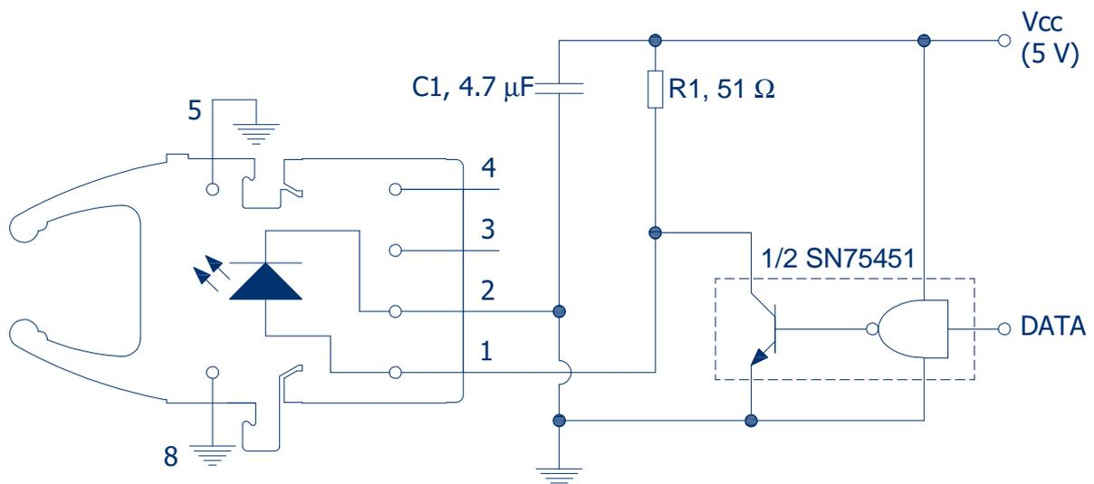
NOTE:  $R1 = 51 \Omega$ , then  $I_F$  drive current is approximately 60 mA. To reduce drive current, select a higher  $R1$  value
