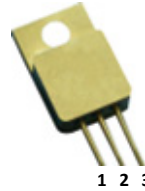
TO – 257 (Isolated Base-plate Hermetic Package)
