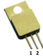
TO – 257 (Isolated Base-plate Hermetic Package)
