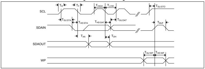
Figure 5-12. Write Cycle Timing
