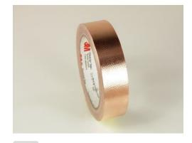
3M™ Embossed Copper Foil Shielding Tape 1245 has a 1.4-mil embossed copper foil backing with acrylic pressure-sensitive adhesive and liner. Embossing makes excellent contact through the adhesive. The unplated copper is for non-corrosive conditions.
