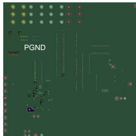
Figure 42f: IRDC3448 Demo board Layout Considerations – Mid Layer 4
