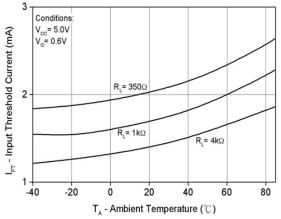
Fig 3 Input Threshold Current vs T<sub>A</sub>
