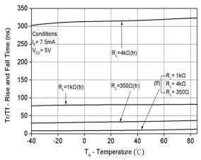
Fig 10 Rise and Fall Time vs T<sub>A</sub>
