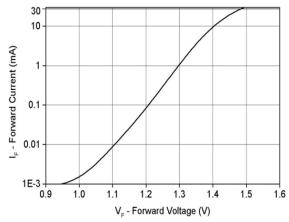
Fig 1 Forward Current vs Forward Voltage
