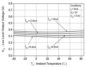
Fig 4 Low Level Output Voltage vs T<sub>A</sub>
