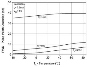
Fig 9 Pulse Width Distortion vs  $T_A$
