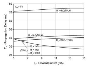
Fig 7 Propagation Delay vs Forward Current
