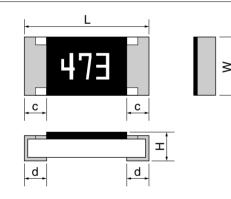
Rated resistance value marking is with 3-digit (E24) or 4-digit (E96) on the over coating. RGC1/16 : only 3digit marking is available. RGC1/16S,1/20 : only No marking is available.
