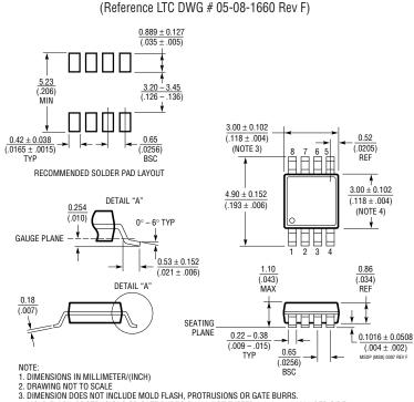
**MS8** Package 8-Lead Plastic MSOP
