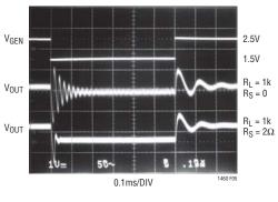
Figure 5. Effect of  $R_S$  for  $C_L = 1\mu F$
