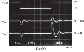
Figure 8.  $C_L = 0.01 \mu F$
