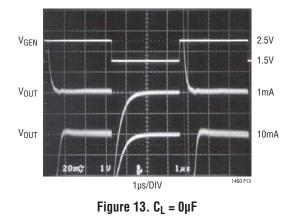
1mA and 10mA load steps with no load capacitance, and Figure 14 shows a 1mA and 10mA load step with a 0.1 $\mu$ F output capacitor. Figure 15 shows the response to a 1mA load step with C<sub>L</sub> = 1 $\mu$ F and 4.7 $\mu$ F.
