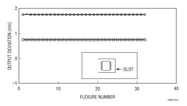
Figure 21a. Same Two LT1460S8-2.5s in Figure 16a, but with Slots
