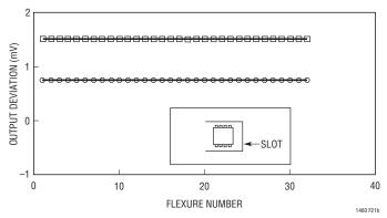
Figure 21b. Same Two LT1460S8-2.5s in Figure 16b, but with Slots
