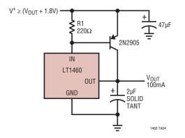
**Boosted Output Current with Current Limit**
