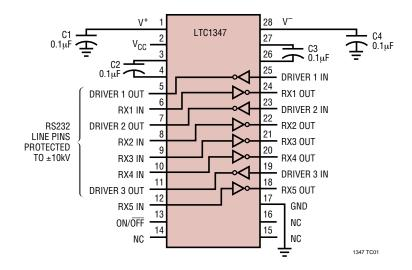
Figure 5. ESD Test Circuit
