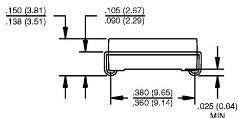
**NOTE:** 1. All dimensions in inches (millimeters)  $\frac{\text{MAX}}{\text{MIN}}$  or typical where noted.
