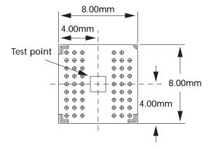
Figure 37: Example Temperature Test Point Location, 90-Ball VFBGA: Top View
