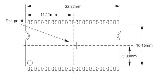
Figure 36: Example Temperature Test Point Location, 54-Ball VFBGA: Top View
