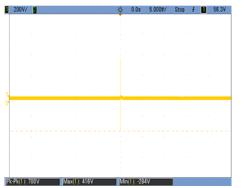
Output voltage waveform(0.41KV)
