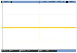
Output voltage waveform(0.42 KV)
