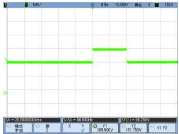
Output voltage waveform(161V/20ms)
