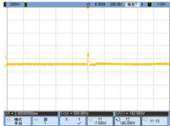
Output voltage waveform (Differential mode 192V)
