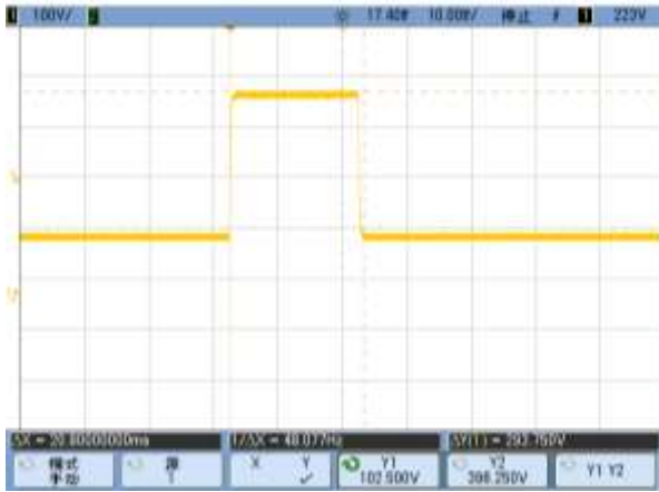
Input voltage waveform (385V/20ms)
