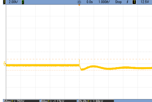
Output voltage waveform (0.75KV)
