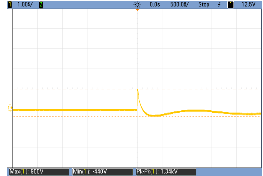
Output voltage waveform (0.9 KV)
