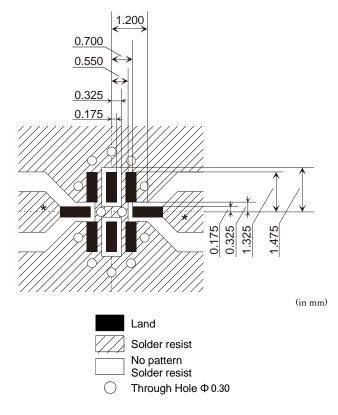
\*Line width to be designed to match  $50\Omega$  characteristic impedance, depending on PCB material and thickness.
