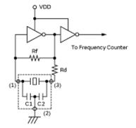
Regarding CERALOCK<sup>®</sup> with built-in capacitors, the terminal (1) and (3) are interchangeable, but if connection is interchanged, the specification of initial tolerance frequency may not be guaranteed. \*Please see dimensions about terminal numbers.
