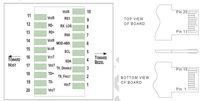
Pin out of Connector Block on Host Board
