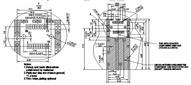
Recommended Front Panel Layout Opening for LC
