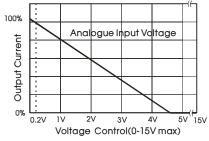
Fig. 10 Analogue input voltage and output current
