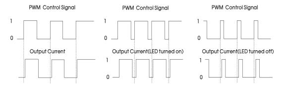
For PWM dimming signals with a certain frequency, the output current of the driver is related to the duty ratio of PWM signal. Refer to the formula for the calculation method:
