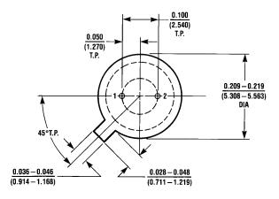
Order Number LM113H, LM113H/883, LM113-1H, LM113-1H/883, LM113-2H, LM113-2H/883 or LM313H NS Package Number H02A
