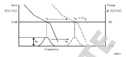
FIGURE 4. Open Loop Response Bode Plot
