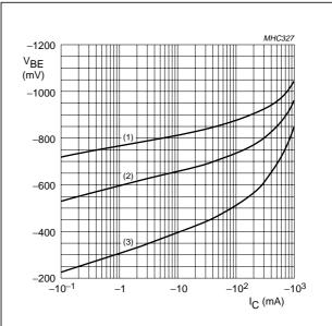
**TR2 (PNP)**  $V_{CE} = -1 \text{ V}.$
